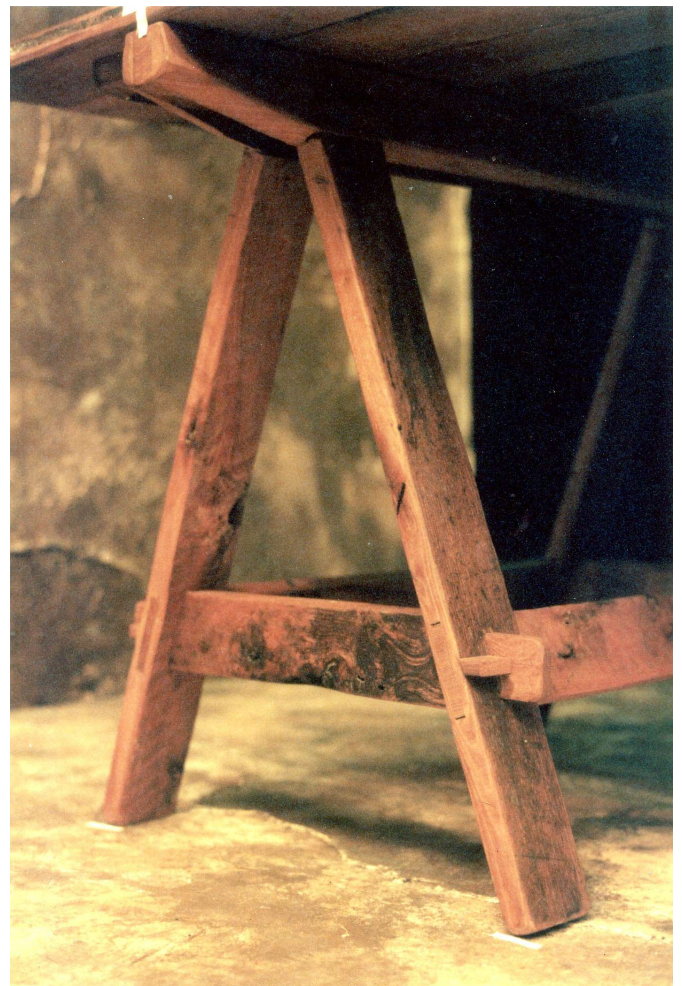
Below: trestles in reclaimed elm. We recently had these back in the workshop after they had been damaged in a fire whilst in storage. A good wash and some attention to the tusk tenons, and they were as good as the day we made them
